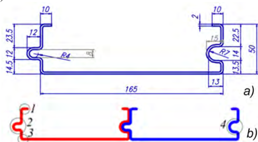
Fig. 1. Profile 165×50×2 mm (a) and assembly pattern (b): 1-4 - areas to be precise enough to allow the construction assemblage
