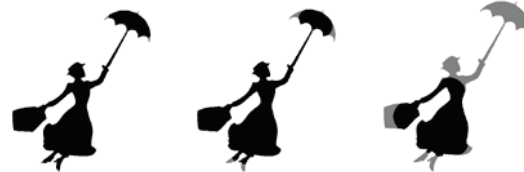
Fig. 2 Decreasing contact areas during the detachment process for a of flat-ended indenter in the form of Mary Poppins.
