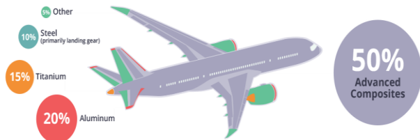
Fig 1. Composites in the Boeing 787's airframe [2]
